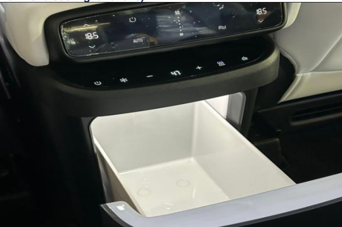
Fig. 16: Xpeng's X9 interior (mini refrigerator – supporting for both warm and cooling functions)
