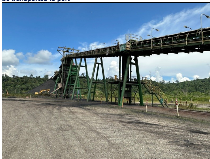
Fig. 6: Conveyor belt to temporary stockpile at Indominco – ready to be transported to port
